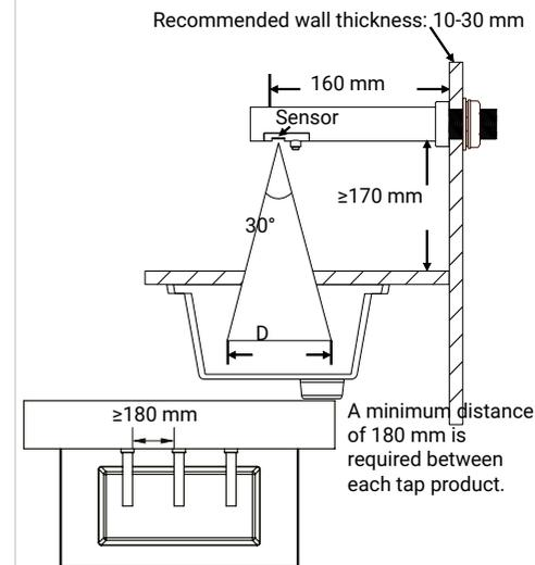
2. Mark the desired position on the wall and drill a  $\varnothing 35$  mm diameter hole.
