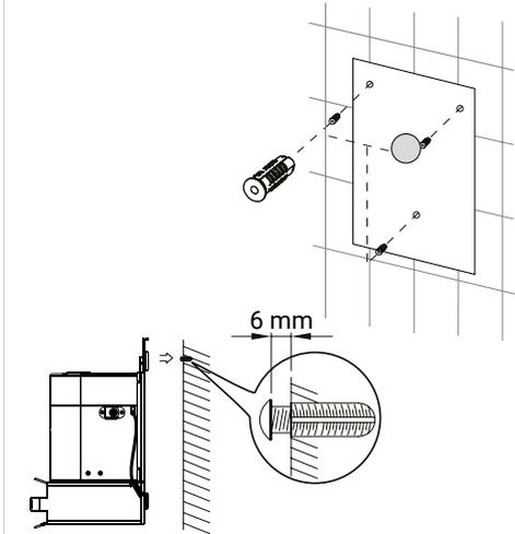
5. Fasten bracket into the pre-drilled holes.
