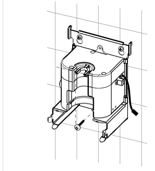
6. Connect the soft rubber tube to the outlet of the pump, and place the pump into the soap container.
