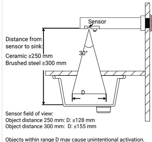
1b. Check the required distance from sensor to sink.
